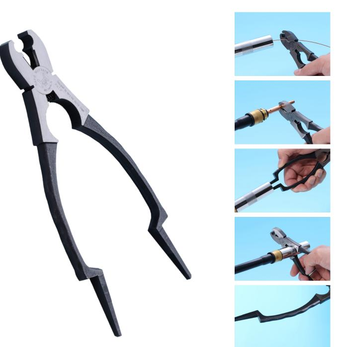
Cleaner pliers for exclusive use of automatic and semiautomatic CO2 welders. Drawing and cutting of wire, desorption of tip, desorption of nozzle, Spatter removal from in and outside the nozzle. Nozzle and insulating cylinder removal and installation. Convenient for robot welding machine. The grip it is easy to hold.
